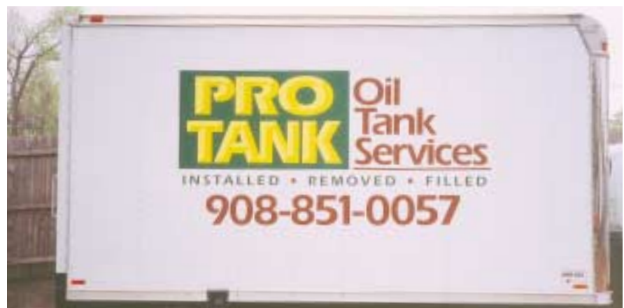
Pro Tank uses a yellow base and lemon yellow highlight. I applied lemon yellow right on the weeded yellow, and then masked the lettering. This allowed me to apply the completed lettering without worrying about the rivets on the truck body throwing off the registration for the highlight.
