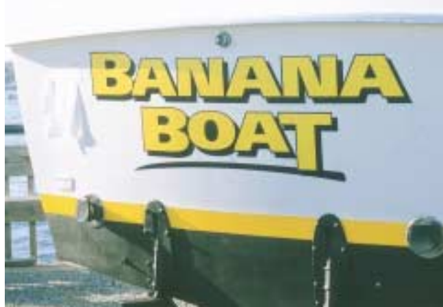
Figure 14. Next, the dark yellow lettering is applied.
