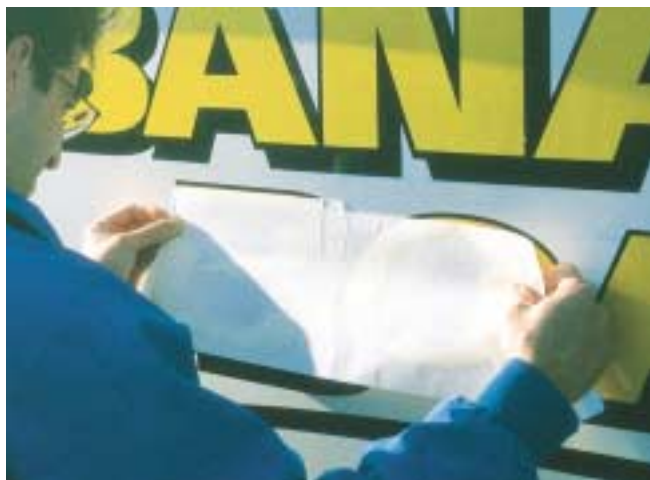
Figure 15. To apply the highlighting color, line the top up with the corners of the lettering.
